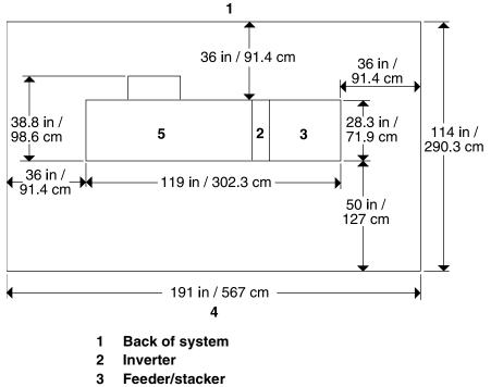
Figure 6-3. 96 with inverter feeder/stacker configuration
